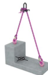
Asymmetrical load: Centre of gravity off-centre
