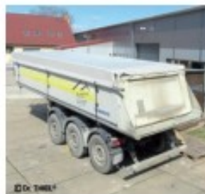
Schmitz - tipper trailer with roll tarpaulin
