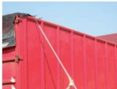
lateral fixing of the tarp by using rubber rope and hook
