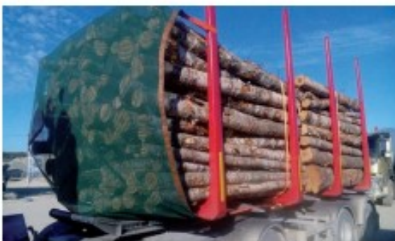
front wall protection in use
