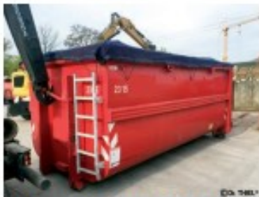
container sheet on a roll-off container
