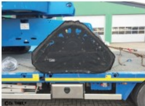
excavator chain protection in pyramid shape
