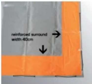
reinforced surround in detail
